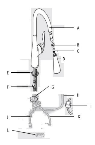
Note: This is for all faucets (10010C, 10011, 10022, 10024) with a pull-out spray, if a fountain faucet is installed he F, H and I are not needed for installation.
