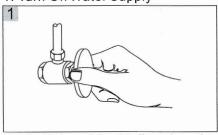
You should clean all the dirts from valve outlets. Turning off the water supply valves. This is usually found near the water meter. If you are replacing an existing faucet, remove the faucet from the sink and clean the sink surface thoroughly.
