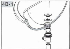
As shown. Insert Flange with Washer through Sink drain Hole. Erom underside, thread Drain Body into Flange. Holding the drain body in position with Ball Rod Opening facing back, tighten Metal Locknut securely. Thread Drain Tailpiece into Drain body.
