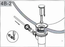
As shown. Place the Drain stopper into the drain body from the top rear. Slide the ball rod into the Ball Rod Opening through Stopper Hole, and threaded it on to the Drain Body.
