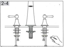
From underneath sink, tighten Mounting Nut by Hand. Before final tightening, make sure Valve Body Side Co]nnector facing Spout Body.
