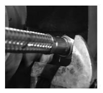
**Step Nine** – Reconnect the water line to the quick connect for the spray wand
